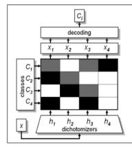
ECOC coding design for a 4-class problem. White, black, and grey positions corresponds to the symbols +1, -1, and 0, respectively. Once the four binary problems are learnt, at the decoding step a new test sample X is tested by the n classifiers. Then, the new codeword  $x = \{x_1, ..., x_n\}$  is compared with the class codewords  $\{C_1, ... C_4\}$ , classifying the new sample by the class  $c_i$  which codeword minimizes the decoding measure.
